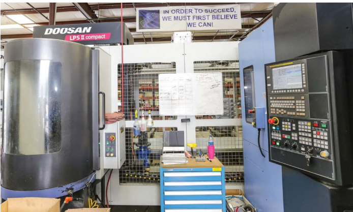
PNM have two Matsuura Hplus300s with 36 pallets, 3 Kiwa KH4500 with 6 pallets each and a Doosan 12 pallet machine. Having multi pallet systems helps minimize parts sitting on their shelves. Activate the job, call up the pallet and away they go. It is pretty common for PNM to get the order in the morning and have the parts out for plating in the afternoon. JIT all the time.
