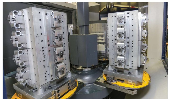
PNM have two Matsuura Hplus300s with 36 pallets, 3 Kiwa KH4500 with 6 pallets each and a Doosan 12 pallet machine. Having multi pallet systems helps minimize parts sitting on their shelves. Activate the job, call up the pallet and away they go. It is pretty common for PNM to get the order in the morning and have the parts out for plating in the afternoon. JIT all the time.
