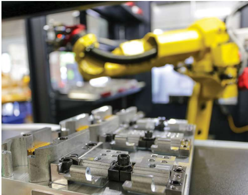
PNM just added a new Trinity robotic cell system attached to a Haas VF2ssYT with 42 tools. Mario estimates that with all 56 pallets populated that they will net 12-14 hours of run time with only three man hours of labor. PNM considers Mexico and China as their biggest competitors so any time they can see long production runs with low labor interaction they are very happy. Pallets, technology, robots, and automation keeps them competitive.
