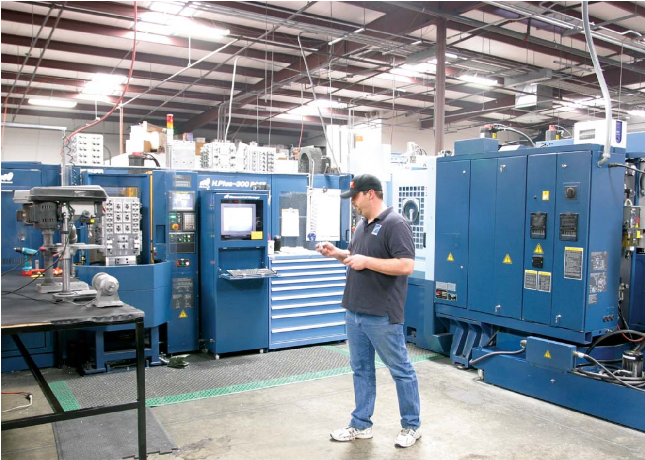
Mario Periscone, tooling shop manager/programmer, checks a part in preparation for scheduling the cell controller on the 17-pallet Matsuura H.Plus 300, 4-axis horizontal. The system has a 20-hp, 15,000-rpm spindle and a 240-tool automatic changer.
